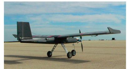
Using SolidWorks Premium software and a Stratasys Dimension FDM 3D printer, SelectTech GeoSpatial built and flew a UAV made almost entirely of 3D-printed parts.
